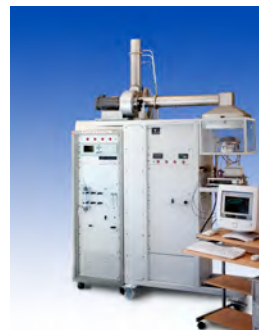
Currently-made, commercial Cone Calorimeter (FTT, London)
