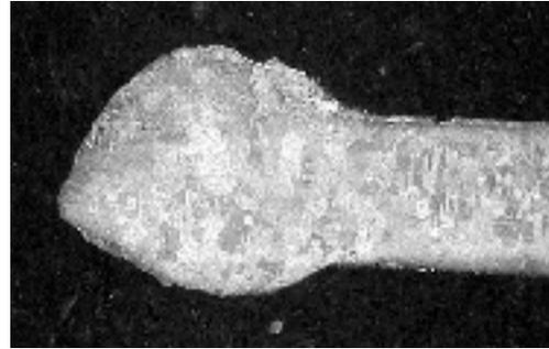
**Figure 2** Bead created by experimental arcing—cross-section view
