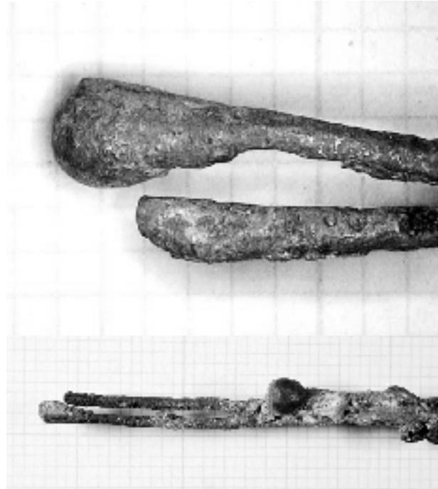
**Figure 5** Examples of melted copper wire beads caused by exposure to fire without arcing
