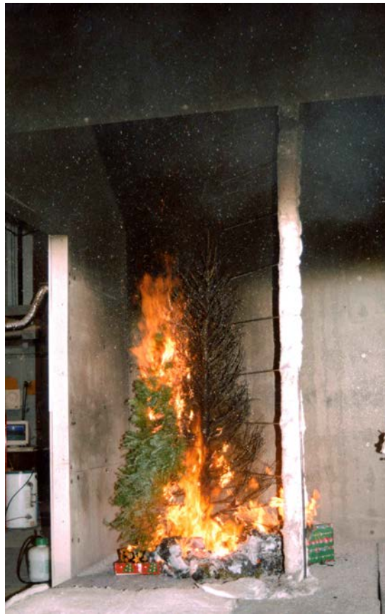
Figure 5 This Christmas tree would not burn when a small flame was applied to a tree branch. Applying the same flame to a small stuffed animal hung on the tree ignited the toy and the tree. Peak HRR = 525 kW.
