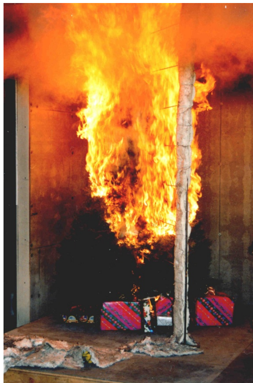
Figure 2 Fierce burning from a dry (MC = 11%) tree. Peak HRR = 2700 kW.
