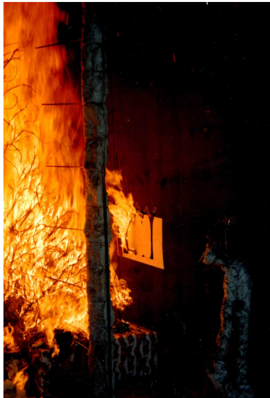
Figure 4 A rapidly burning tree will ignite nearby combustibles. Here nearby fabric targets are shown being ignited.
