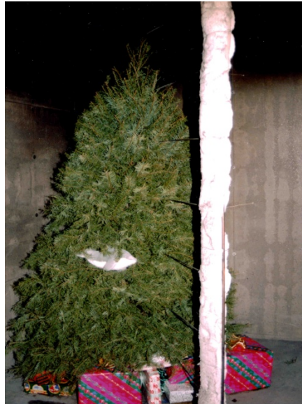
Figure 1 An example tree ready for testing. All test trees included gift packages under the tree and a single stuffed toy animal in the middle of the tree. Ignition was by small flame to a branch; or by small flame to stuffed toy; or by small flame to gift packages. No tree failed to burn from at least one of these ignition locations.
