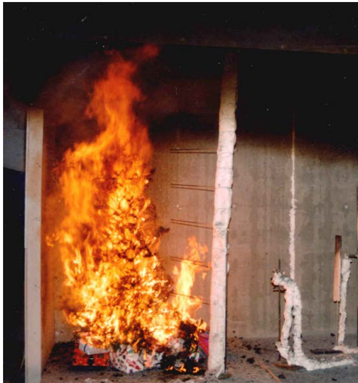
Figure 7 This FR-treated tree burned vigorously and essentially burned up completely.
