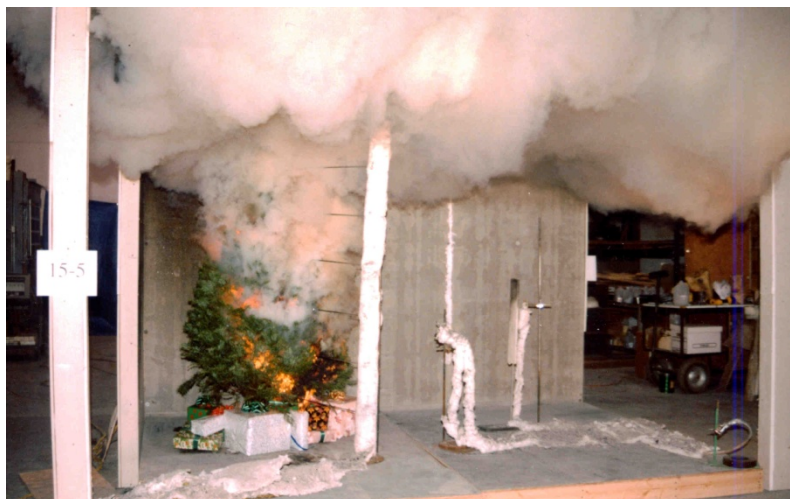
Figure 6 A fire-retardant tree burning. Some FR specimens generated a great deal of mist.
