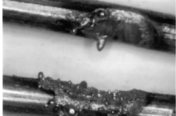
Figure 4. Arc beads with an irregular shape (obtained in laboratory testing by making direct contact between uninsulated conductors carrying 240 VAC) (Courtesy David Reiter).
