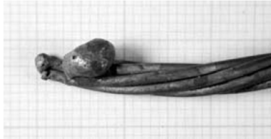
Figure 3. ‘Victim’ bead from a real fire (Courtesy Yasuaki Hagimoto).
