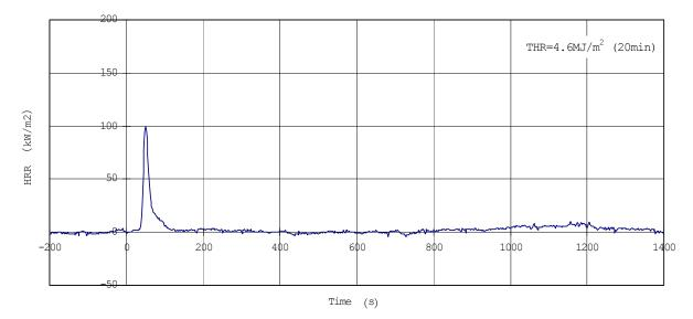
Fig.3 Heat release rate curve (Specimen : Decorated gypsum board)
