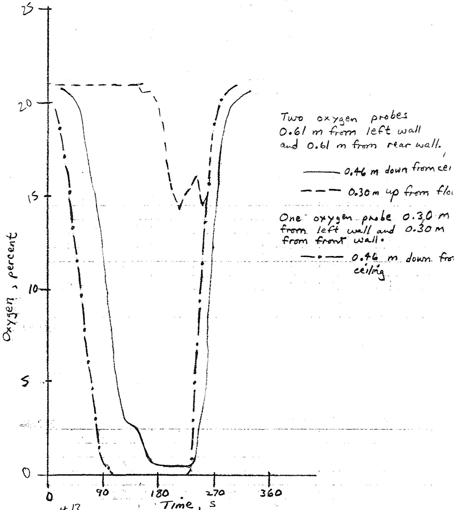
Fig. #13. Oxygen concentrations in room for test 19 (plywood 2, exposure A)
