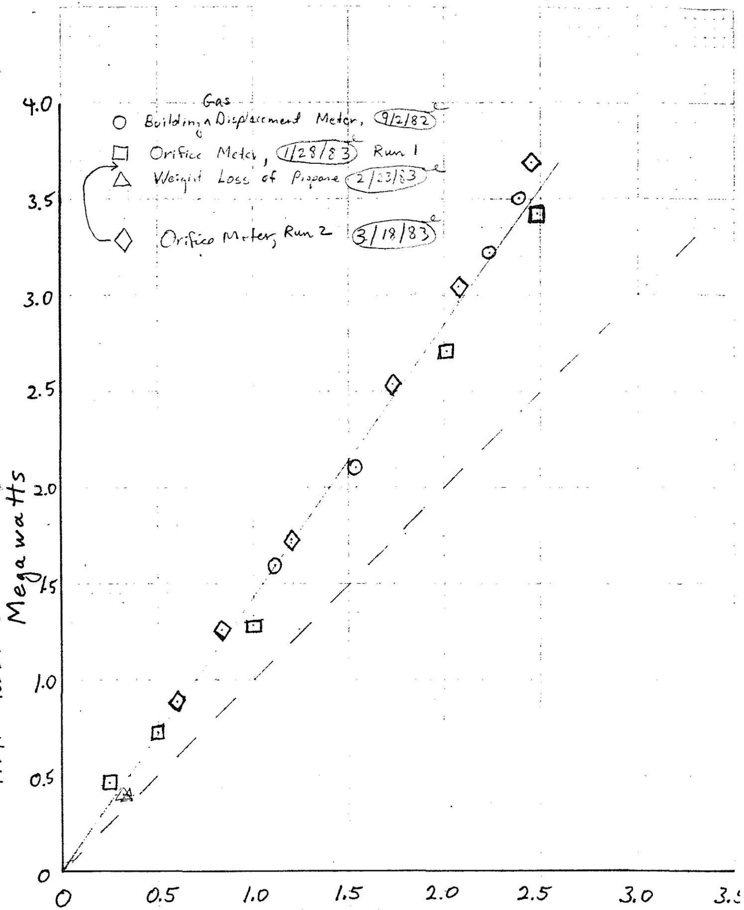
NET HEAT RELEASE RATE BY GAS FLOW TO BURNER
