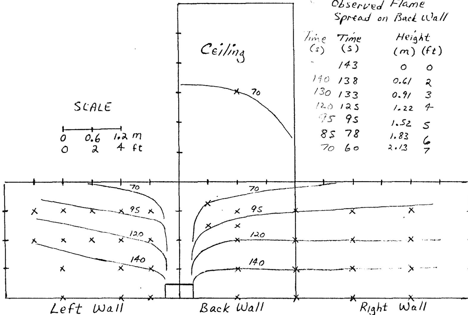
x - Placement of surface thermocouples
