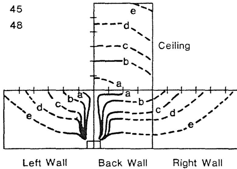
Fig. 8 Flame spread profiles for test 10 (polystyrene, exposure A)
