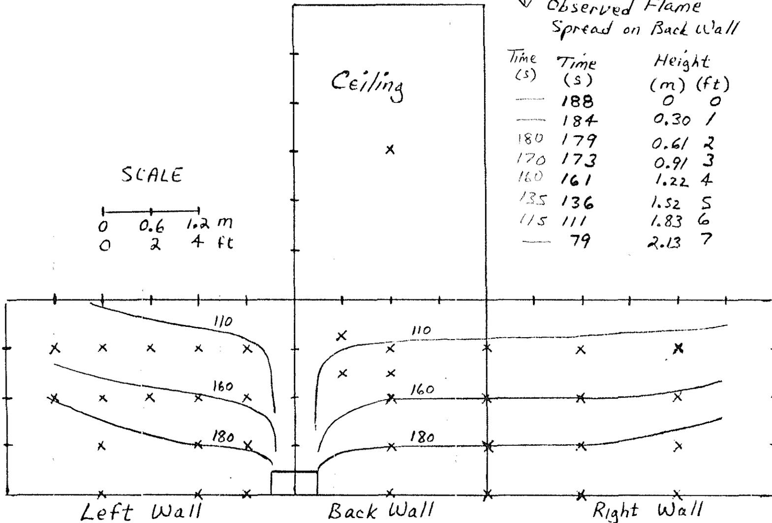
x - Placement of surface thermocouples
