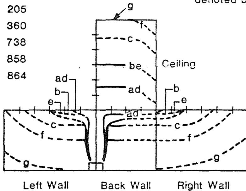
Fig. 17 Flame spread profiles for test 15
