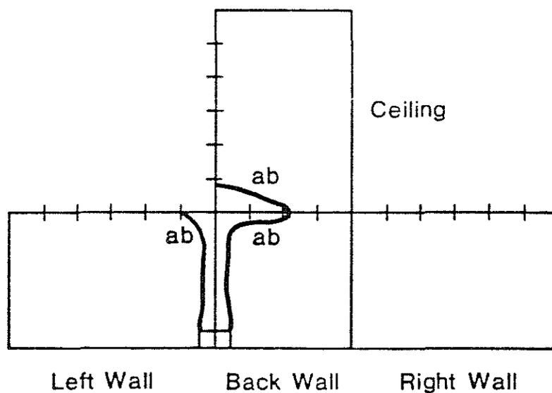
Fig. 7<sup>A6</sup> Flame spread profiles for test 1B
