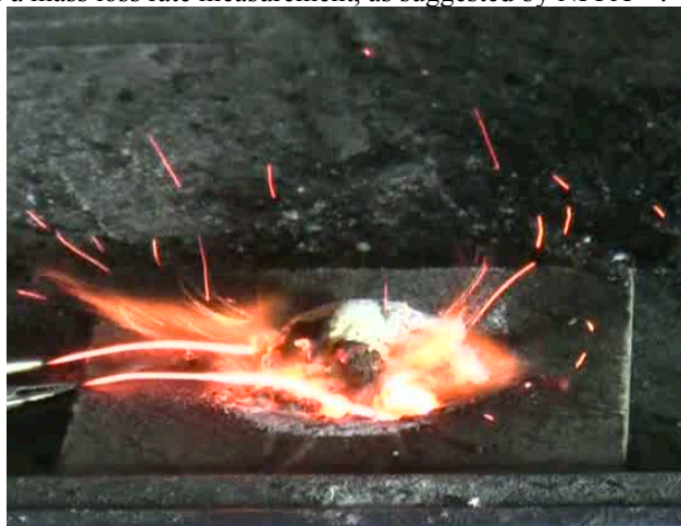
Figure 3 Ammonium nitrate being tested in the UN Test O.1 (photograph by author)
